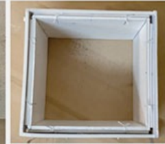
In 3rd configuration all the Blinds are perfectly flushed within gaps
